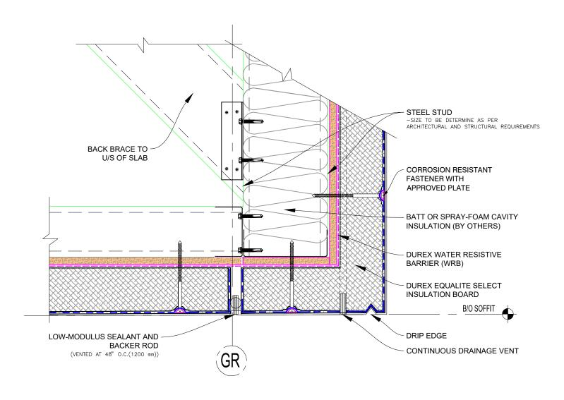
Durabond details are offered to assist in the development of project specific details. Design principles and variables incorporated in the final details and specifications are the responsibility of the project design professional.
